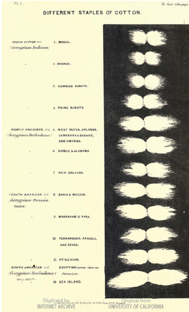
FIGURE A.8.—Length of cotton staples for various cotton types. Reproduced from Wheeler (1862).
