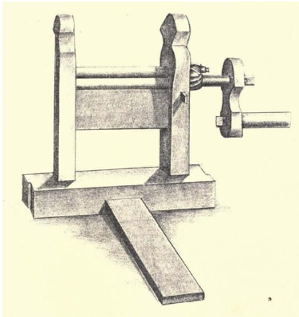
FIGURE A.3.—Indian Churka for removing cotton seeds. Reproduced from Wheeler (1862).
